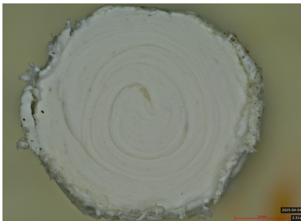
Figure 1. Optical microscopy image showing the cross-section of the extruded HDPE-PLA-TiO 2 composite filament.
