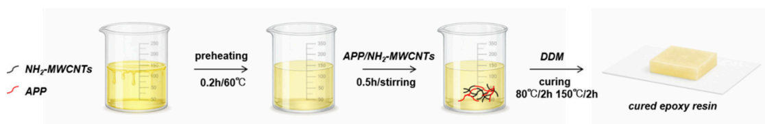
Figure 2. Preparation process of cured epoxy resin.
