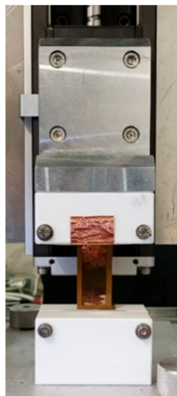
Figure A2. Picture of the Festo mechanical slide with clamps for EH tests.
