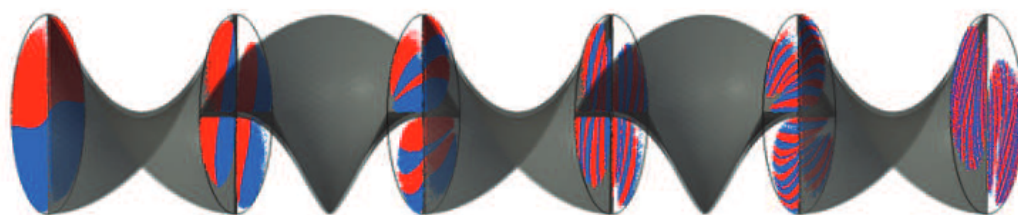
Figure 6. Two particle clouds (red and blue) within a fluid domain exemplary of a kenics mixing element illustrate the interface between the clouds at the inlet ( \lambda_0 ) and outlet ( \lambda_1 ), where \lambda_0 < \lambda_1 applies. The flow direction is from left to right [9].
