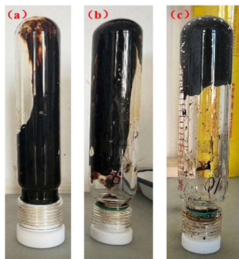
Figure 17. Gelation state of thixotropic gel system after aging for 7 days at different temperatures: (a) 120 °C; (b) 130 °C; (c) 140 °C.
