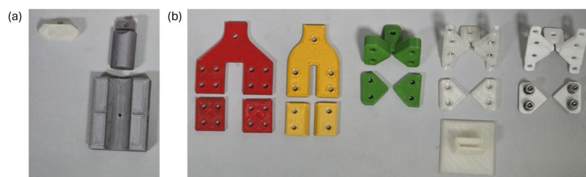
Figure 2. Example of some of the different clamps designed and FDM manufactured in PLA. Each group has its own clamping strategy: (a) adhesive clamping; (b) mechanical clamping. Different colors were used to visually reinforce that different versions of clamps were studied.
