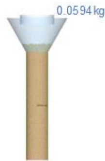
Figure 12. Direct bulk density measurement in test simulation.
