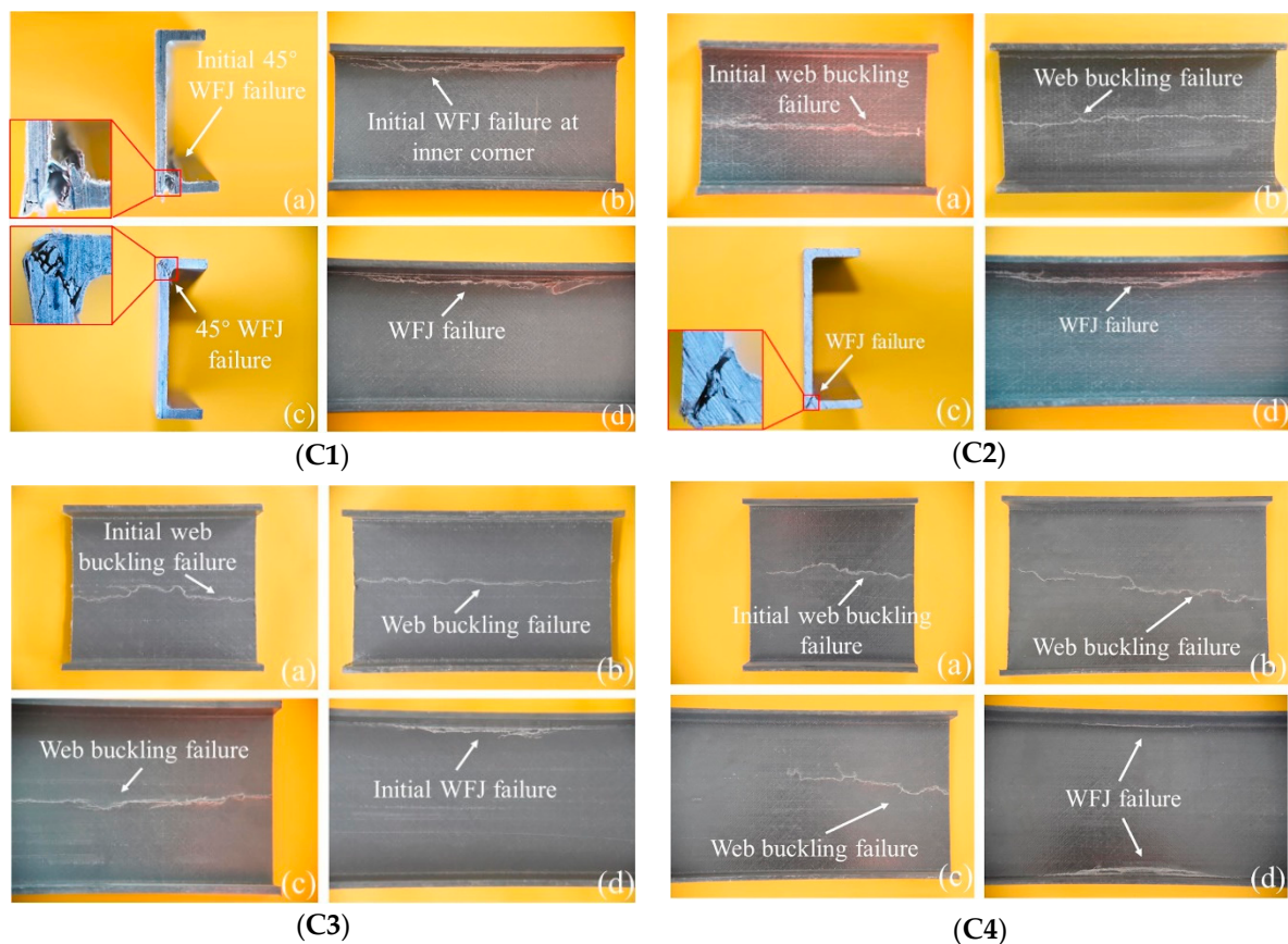
Figure 9. Observed failure modes of channel sections conducted by Wu et al. [20].
