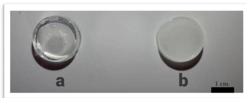
Figure 3. Macrophotographs of the PEGMA11/PEGDA11 (a), and PEGMA11/PEGDA11/f-PVA3 (b) hydrogels.
