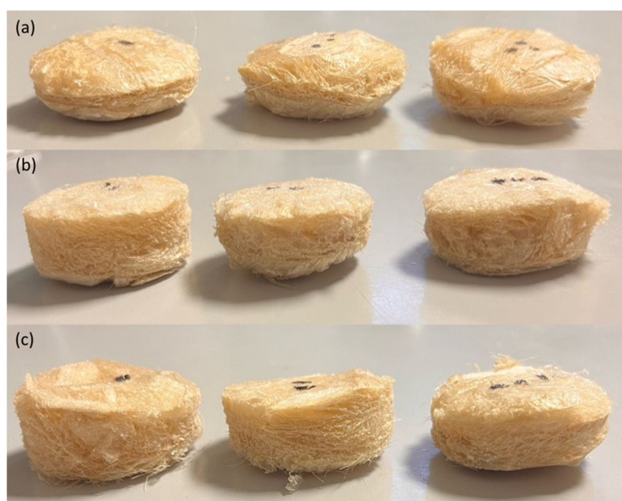
Figure 1. Images of soy protein isolate (SPI) biocomposites prepared with spent coffee grounds (C) by freeze-drying with a sheep wool content (W) of (a) 10, (b) 15, and (c) 20 wt%.
