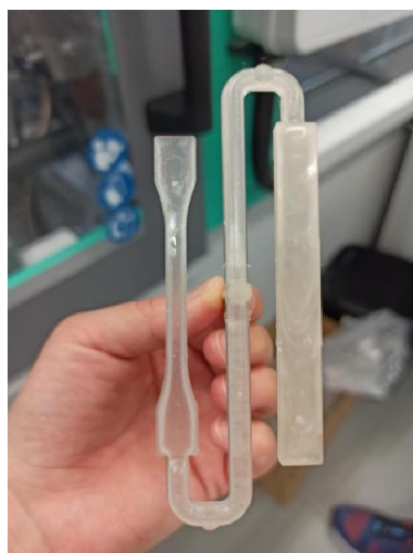
Figure 1. The item obtained by injection molding dedicated to the testing of mechanical properties of the material.
