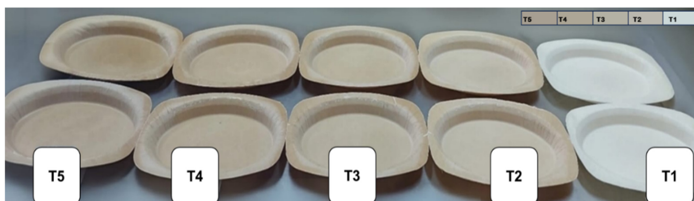
Figure 2. Foam trays developed from brewer's malt bagasse flour (A) and potato starch (B) in different formulations. T1: 100%B, T2: 10%A + 90%B, T3: 20%A + 80%B, T4: 30%A + 70%B and T5: 40%A + 60%B.
