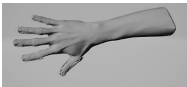
Figure 3. Scan of the hand and part of the forearm using an EinScan PRO HD SHINING 3D scanner. Point image.
