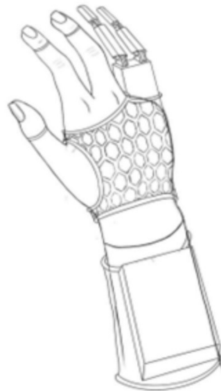
Figure 1. Schematic drawing showing a first concept of a control module on the forearm with a microcontroller placed in the housing.
