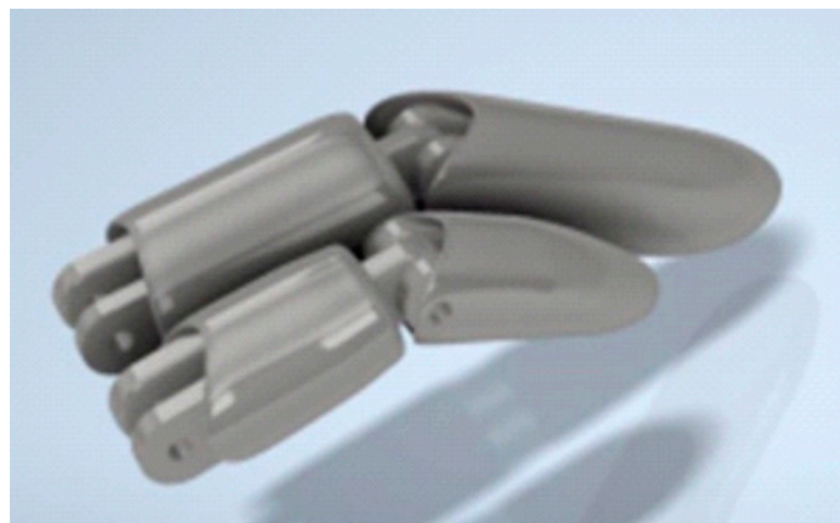
Figure 5. Model of missing parts of fingers based on the dimensions and shape of a human hand, designed in AUTODESK Inventor 2025.
