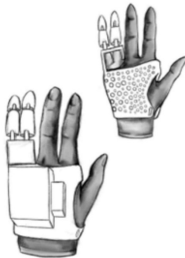
Figure 2. Schematic drawing showing a second concept of a control module on top of the hand, with a microcontroller placed in a box.
