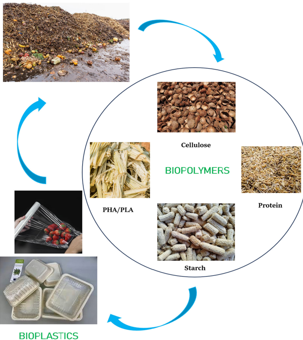
Figure 11. Flowchart illustrating the transformation of agricultural waste into biopolymers for food packaging.
