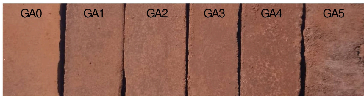
Figure 8. Image of the samples and the colour variation in the geopolymer due to the addition of FAN in its matrix. From left to right, GA0, GA1, GA2, GA3, GA4, and GA5 family.
