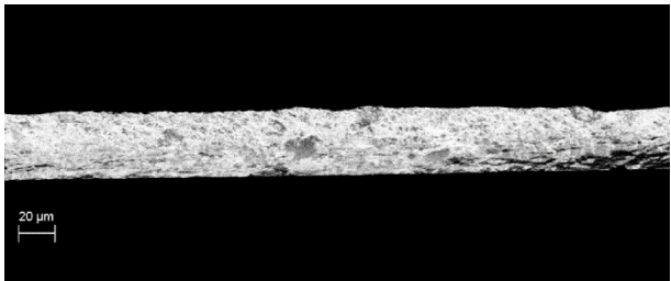
Figure S1. SEM image of PTBr film cross section.
