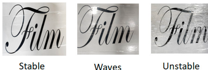
Figure 7. Photographs of multilayer films: visualization of a stable film, wave-like instabilities, and the presence of defects.
