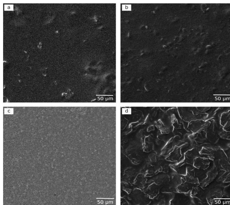
**Figure 2.** Scanning electron microscopy (SEM) images of (a) Alg/rGO<sub>4.5</sub>, (b) Alg/rGO<sub>9</sub>, (c) Alg/TA<sub>9</sub>, and (d) Alg/rGO<sub>4.5</sub>/TA<sub>9</sub>.
