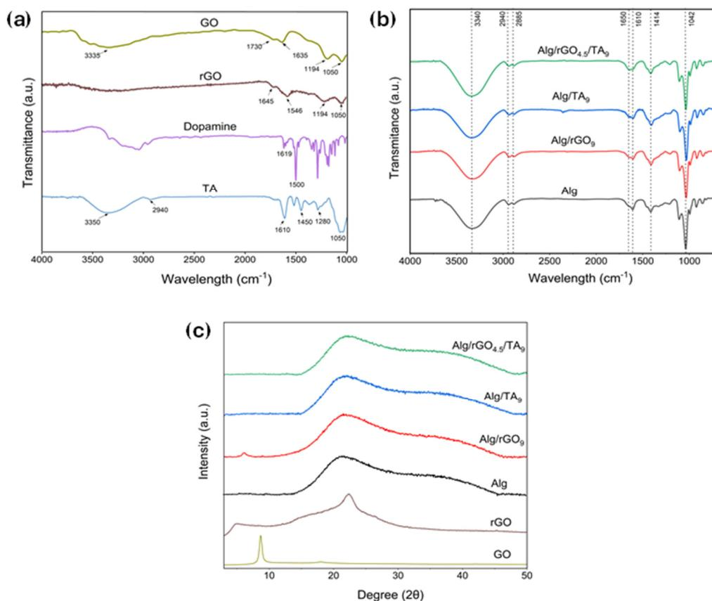
**Figure 3.** (a) FTIR spectra of GO, rGO, DA, and TA; (b) FTIR spectra of Alg, Alg/rGO<sub>9</sub>, Alg/TA<sub>9</sub>, and Alg/rGO<sub>4.5</sub>/TA<sub>9</sub>; (c) XRD spectra of GO, rGO, Alg, Alg/rGO<sub>9</sub>, Alg/TA<sub>9</sub>, and Alg/rGO<sub>4.5</sub>/TA<sub>9</sub>.
