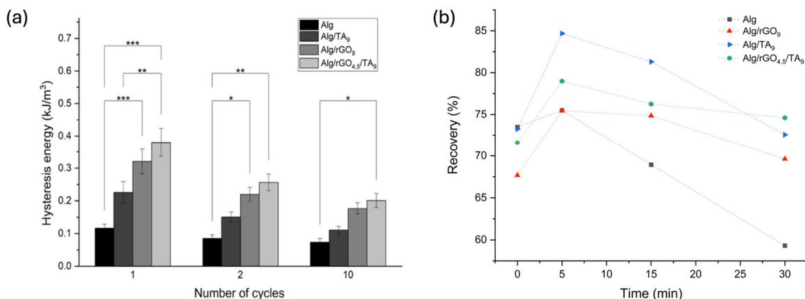
**Figure 5.** (a) Hysteresis properties of Alg hydrogels with different rGO and TA contents. (b) Self-recovery properties of Alg hydrogels with different rGO and TA contents. (\*)  $p \leq 0.05$  (\*\*)  $p \leq 0.01$  and (\*\*\*)  $p \leq 0.001$ .
