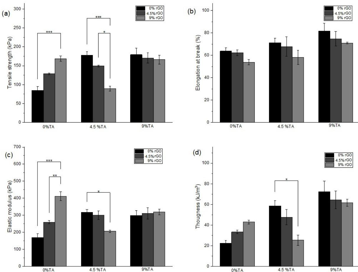
**Figure 4.** Mechanical properties in tensile tests including (a) tensile strength, (b) elongation at break, (c) elastic modulus, and (d) toughness for Alg hydrogels with different rGO and TA contents. (\*)  $p \leq 0.05$  (\*\*)  $p \leq 0.01$  and (\*\*\*)  $p \leq 0.001$ .
