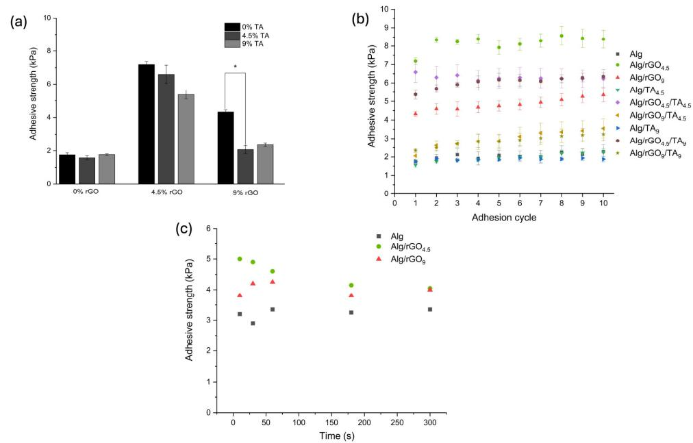
**Figure 6.** Adhesive properties of hydrogels with different rGO and TA contents in pigs skin, including (a) the corresponding adhesion strength, (b) repeated adhesion of the hydrogels to the substrate, and (c) the effect of hydrogel–substrate contact time prior to separation. (\*)  $p \leq 0.05$ .
