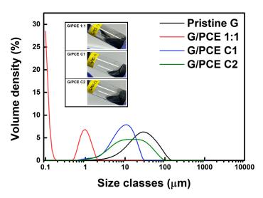
**Figure 5.** Particle size analysis of pristine graphene, G/PCE 1:1, G/PCE C1, and G/PCE C2 dispersions.
