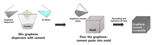
Figure 2. Manufacturing process of graphene–cement composite.
