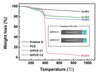
Figure 3. TGA graphs of pristine graphene, pure PCE, G/PCE C1, and G/PCE C2.
