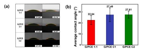
**Figure 6.** (a) Photo images of contact angle measurement of G/PCE 1:1, G/PCE C1, and G/PCE C2 dispersions with cement plate. (b) Average contact angles.
