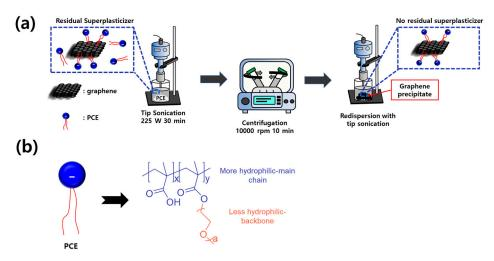
**Figure 1.** (a) Production procedure for G/PCE 1:1, G/PCE C1, and G/PCE C2. (b) Chemical structure of PCE.
