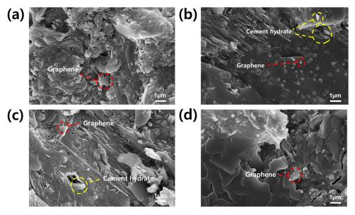
**Figure 9.** FE-SEM images of GCCs made from (a) pristine graphene, (b) G/PCE 1:1, (c) G/PCE C1, and (d) G/PCE C2 dispersions.
