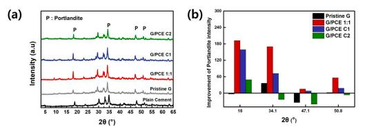
**Figure 8.** (a) XRD analysis of plain cement and GCCs with PCE and (b) peak enhancement degree of portlandite peaks of GCCs compared to that of plain cement.
