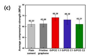
**Figure 7.** Photographs of (**a**) GCC samples made from G/PCE 1:1 dispersion and (**b**) compressive strength test. (**c**) Average compressive strength of GCC samples made from plain cement, pristine graphene, G/PCE 1:1, G/PCE C1, and G/PCE C2 dispersions.
