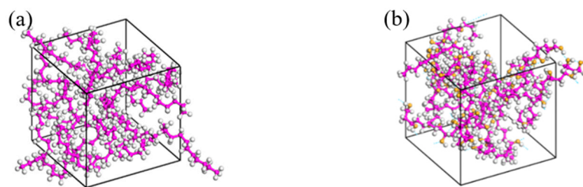
Figure 2. Adsorption cell model: (a) HDPE; (b) EVOH (the white atoms are hydrogen atoms, the purple atoms are carbon atoms, the yellow atoms are oxygen atoms).
