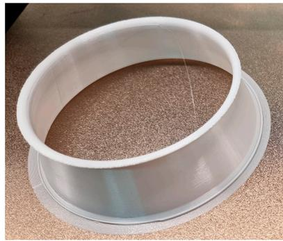
**Figure 14.** The “Coandă Surface element” at the end of the printing process.
