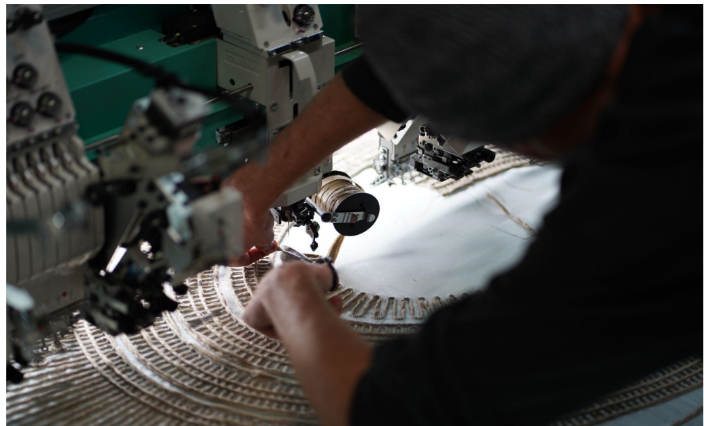
Figure 1. Photograph of tailored fiber placement fabrication production using a Tajima dual headed embroidering machine.
