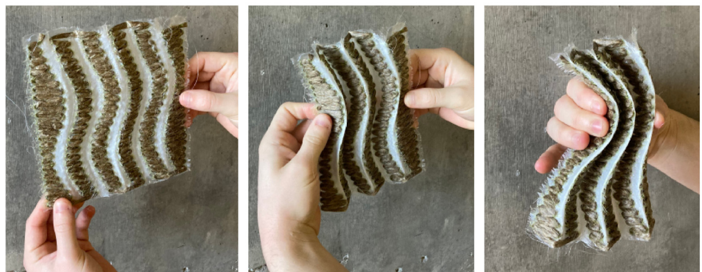
Figure 6. An image sequence of test sample, demonstrating folding along lines created through selective curing.
