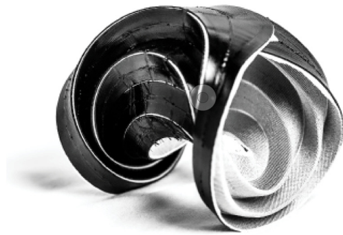
Figure 12. Photograph of final demonstrator made by 3D printing TPU on fabric.
