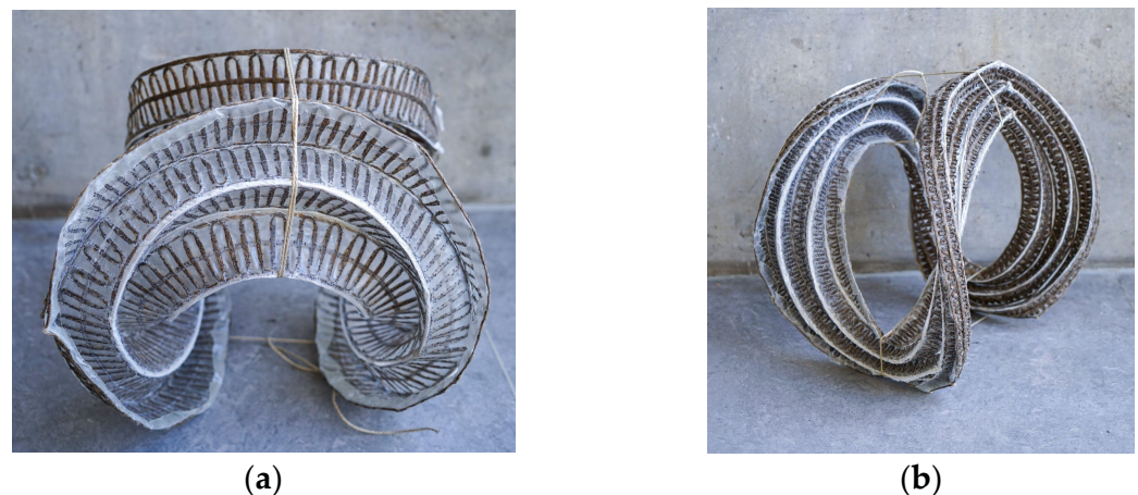
Figure 8. Images of hand bent prototypes furnished to improve methods and design processes. Both prototypes have the same circular outer diameter of 400 mm while testing a variety of other parameters. Prototype (a) contains six 5 mm corrugations with 8 mm folding zones. Prototype (b) contains five 10 mm corrugations with 5 mm folding zones.
