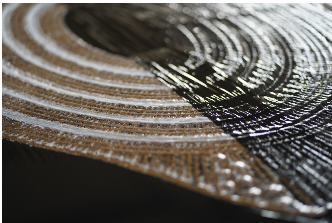
Figure 15. Close up image of a cured flat preform with silicone hinges. During curing, the preform was placed between plastic sheets in a vacuum press table.
