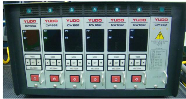
**Figure A3.** Hot runner controller employed in this work for control of the cylinder temperature (CW662, Yudo, Hwaseong, Republic of Korea).
