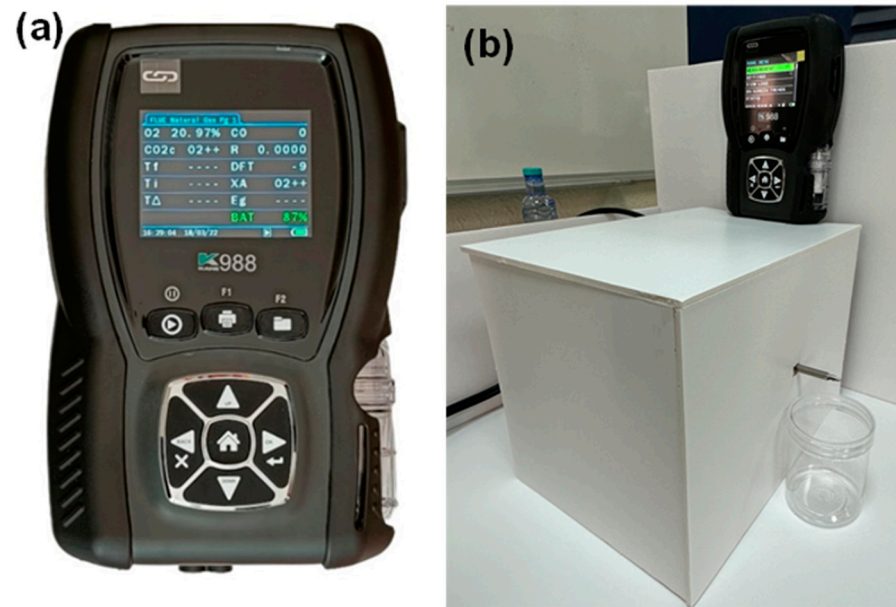
Figure 8. Emission tests on epoxy samples: (a) gas analyzer and (b) test setup.
