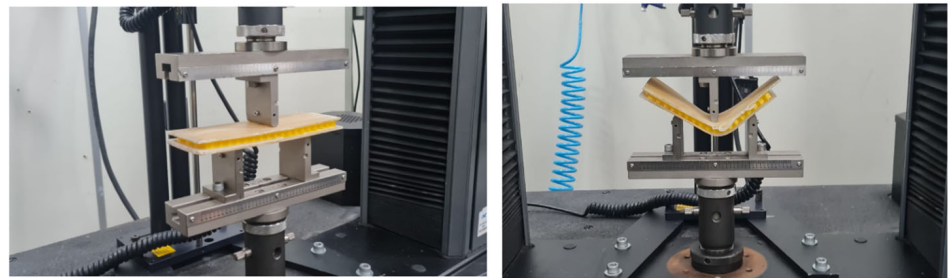
Figure 12. Three-point bending test of specimen 1.
