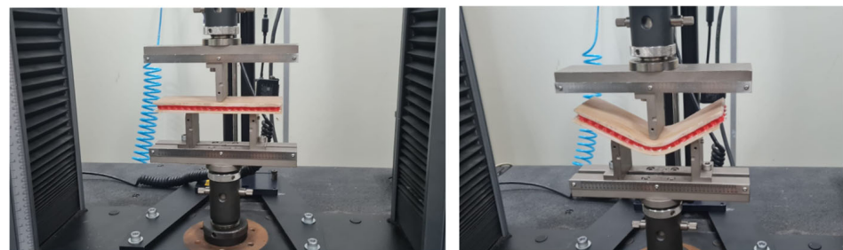
Figure 13. Three-point bending test of specimen 2.
