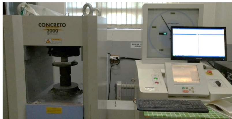
Figure 3. Compressive strength test on samples.
