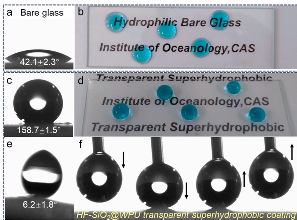
Figure 6. (a) WCA image and (b) optical images of water droplets on bare glass; (c) WCA image and (d) optical images of water droplets on the HF-SiO 2 @WPU superhydrophobic coating; (e) SA image and (f) dynamic water droplet contact behavior on HF-SiO 2 @WPU superhydrophobic surfaces.
