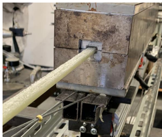
Figure 7. Close up on the pultruded profile during run 2.
