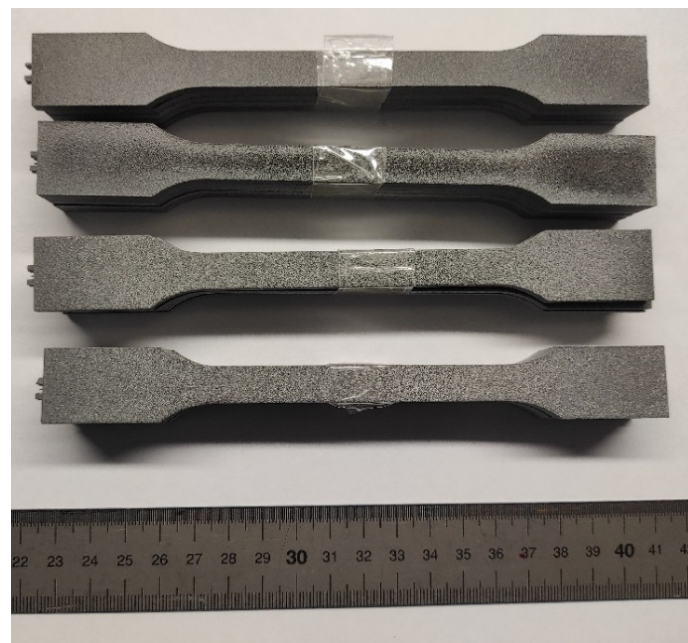
Figure 4. Printed samples for testing under uniaxial tensile loads.
