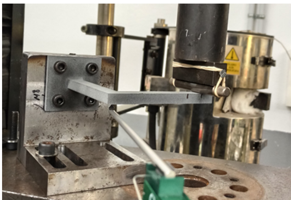
Figure 10. Experimental setup for the mechanical test on printed handles.
