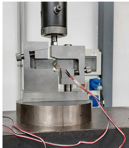
Figure 9. Shear sample mounted on the testing device.
