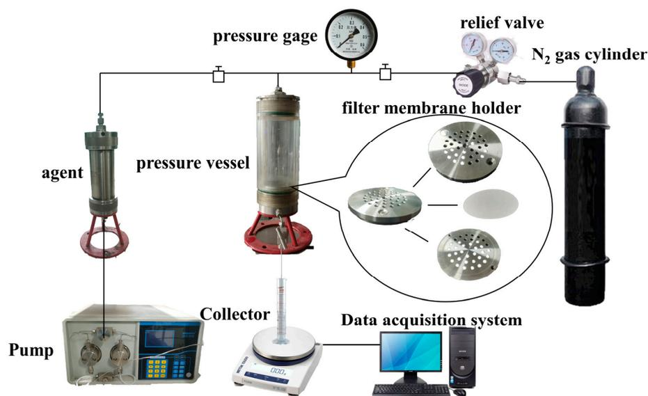
**Figure 1.** Schematic of the microporous membrane filtration experiment.
