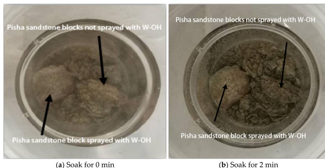
**Figure 1.** Pisha sandstone dissolves in water.
