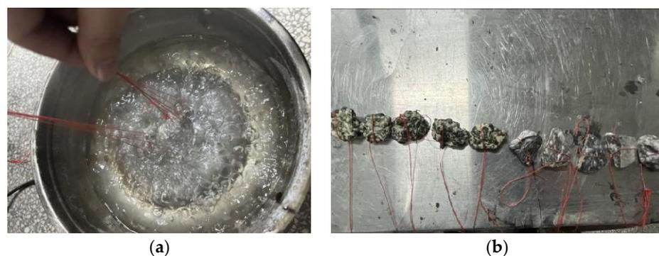
**Figure 3.** Polyurethane binder and aggregate adhesion test. (a) In boiling; (b) after boiling.
