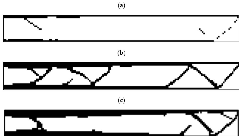
**Figure 11.** The results for the optimization of the rectangular plane in terms of (a) 20%, (b) 40%, and (c) 60% for the weight constraint.
