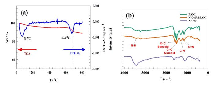
Figure 3. (a) TGA curve of the NiOnF, (b) FT-IR of PANI, NiOnF@PANI, and NiOnF.
