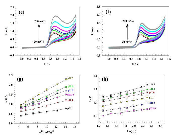
**Figure 7.** CVs of modified electrode GC/PANI/NiOnF at various sweep rate ranges (20 to  $200 \text{ mV s}^{-1}$ ) in 0.5 mM nitrite solution and 0.1 M PBS at different pH ranges (**a**). pH 2, (**b**). pH 4, (**c**). pH 6, (**d**). pH 7, (**e**). pH 8, and (**f**). pH 10). (**g**) The relation between the square root of sweep rate and nitrite's oxidation current. (**h**) The relation between the Log of sweep rate versus nitrite's oxidation potential.
