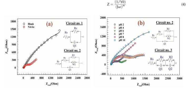
Figure 8. (a) Nyquist plots of modified electrode GC/PANI/NiOnF at constant AC potential of 1.0 V in the presence and absence of nitrite. (b) Nyquist plot of the modified GC/PANI/NiOnF at AC Potential of 1.0 V at different solution pH (2–10). Inset figures: the fitting circuits of the corresponding EIS result.
