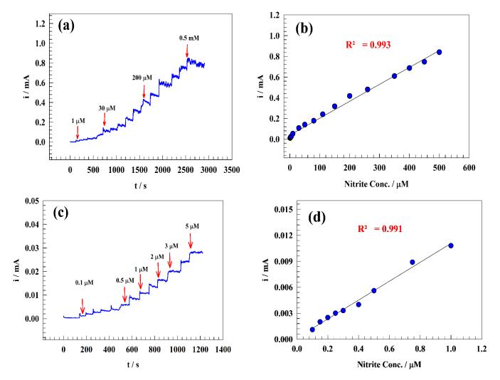
**Figure 9.** (a) Chronoamperogram of sequential addition of nitrite to the drinking water solution, (b) Typical calibration curve of nitrite detection in drinking water. (c) Chronoamperogram of the low concentration range for sequential addition of nitrite. (d) The corresponding calibration curve for low-concentration addition of nitrite ion.
