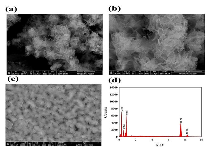
Figure 2. (a,b) SEM images of NiOnF at different magnifications, (c) PANI, (d) EDAX spectrum of NiOnF.
