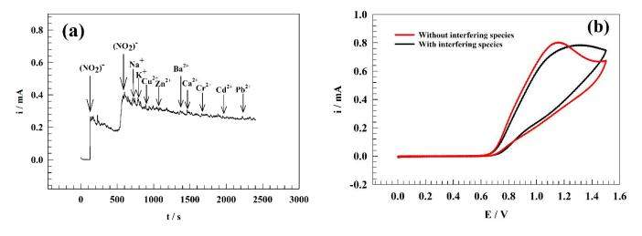
**Figure 10.** (a) Chronoamperogram of the modified GC/PANI/NiOnF electrode in the existence of different interfering ions. (b) CVs of GC/PANI/NiOnF in the presence and absence of interfering species.
