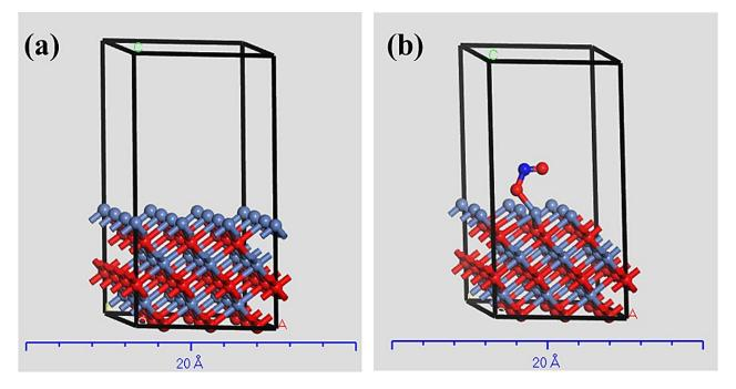
Figure 5. (a) Clean NiO{100} surface, (b)  $NO_2^-$  adsorbed on NiO{100} surface.
