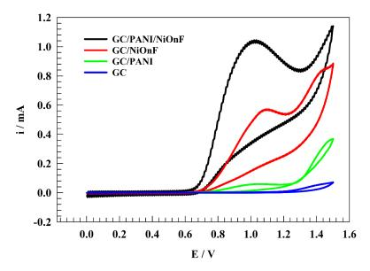
**Figure 4.** CVs of the different electrodes (GC/PANI/NiOnF, GC/NiOnF, GC/PANI and GC) in solution of 0.1 M PBS (pH = 7) and 0.5 mM nitrite at scan rate 20 mV s<sup>-1</sup>.
