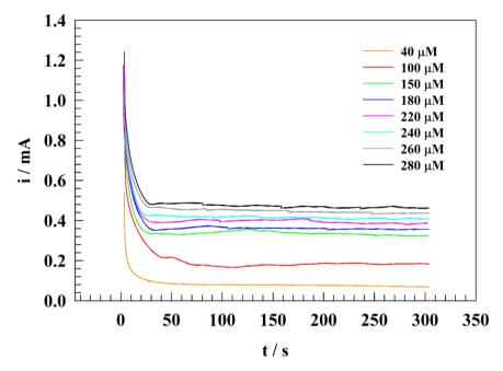
**Figure 11.** Constant potential chronoamperogram for adding different nitrite concentrations in the Nile River water at pH =7 and constant potential of 1.0 V.
