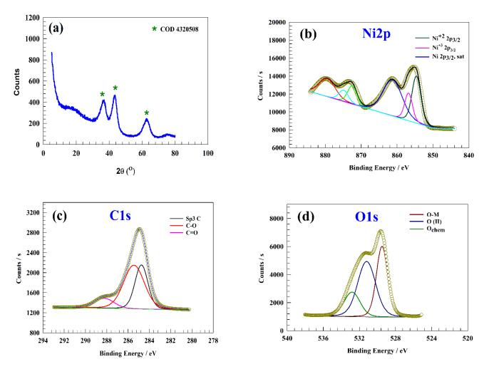
Figure 1. (a) XRD pattern of NiOnF, XPS of NiOnF spectra of (b) Ni2p, (c) C1s, and (d) O1s.
