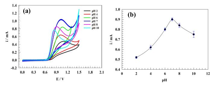
**Figure 6.** (a) CVs of the GC/PANI/NiOnF in 0.5 mM nitrite solution at different pH values. (b) The dependence of oxidation current on the pH of the solution.
