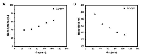
**Figure 4.** Samples are fabricated by using interdigitated electrodes with different gaps. (**A**) The transmittance (@600 nm) of the samples when applying an AC voltage of 80 V between the top and bottom electrodes. (**B**) The reflection bandwidth of the samples in the infrared region when applying a DC voltage of 50 V between the interdigitated electrodes.
