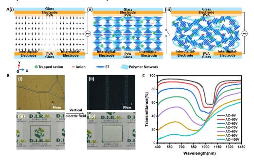
**Figure 2.** (**A**) Schematic diagram of (**i**) the vertical AC E-field between the top and bottom electrodes, (**ii**) the initial CLC cholesteric texture before applying the E-field, (**iii**) the focal conic texture after applying the E-field. (**B**) The POM images of the sample before (**i**) and after (**ii**) applying the E-field. The pictures of the sample before (**iii**) and after (**iv**) applying the E-field. (**C**) Transmittance spectra of the sample under different AC voltages.
