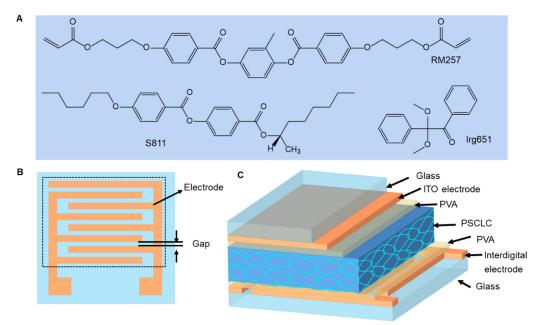
dopant concentration was selected such that the reflection notch of the PSCLC cells was centered at 1050 nm.
