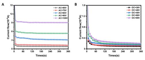
**Figure 6.** Samples fabricated by using the interdigitated electrodes with electrode width 95  $\mu$ m and gap width 25  $\mu$ m. (A) Current flow in the visible light scattering in the presence of different operation voltages. (B) Current flow in the IR broadband reflection in the presence of different operation voltages.
