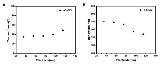
**Figure 5.** Samples are fabricated by using the interdigitated electrodes with different electrode widths. (A) The transmittance (@600 nm) of the samples when applying an AC voltage of 80V between the top and bottom electrodes. (B) The reflection bandwidth of the samples in the infrared region when applying a DC voltage of 50V between the interdigitated electrodes.
