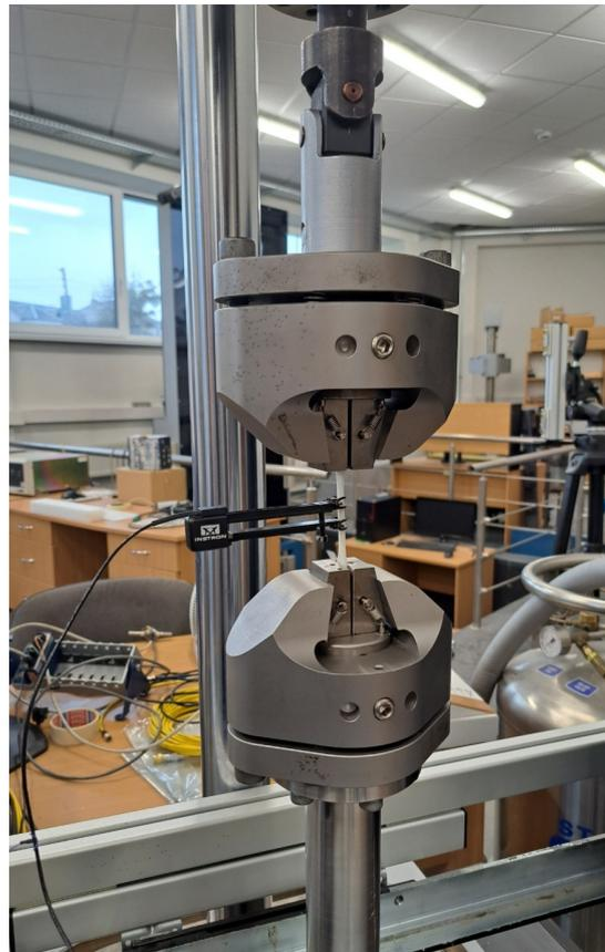
**Figure 3.** Mechanical testing machine: ElectroPuls® E10000 Linear-Torsion.
