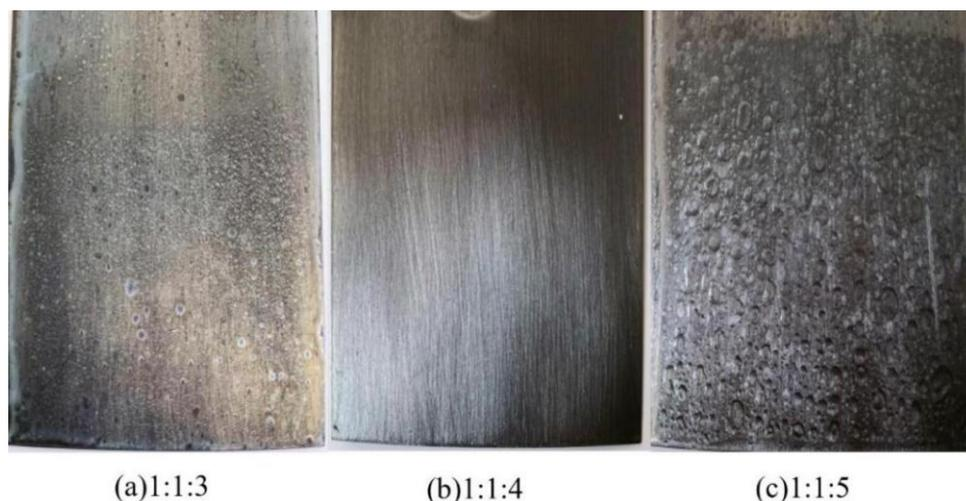
**Figure 7.** Characterization diagram of acid resistance of cured films with different MXDA content (24 h): (a): 1:1:3, (b): 1:1:4, (c): 1:1:5.
