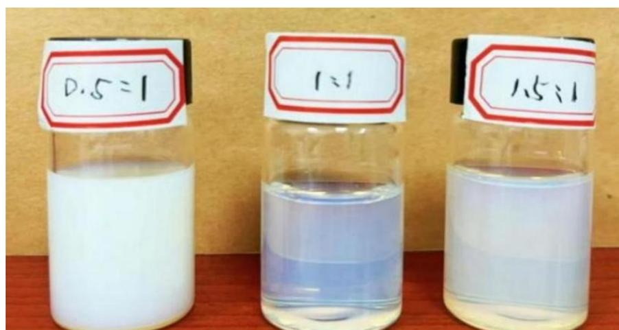
**Figure 4.** The effect of molar ratio of PEG1000 and E20 on the water solubility of curing agents.
