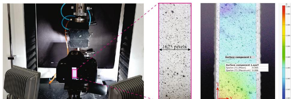
**Figure 4.** DIC setup including imaging and lighting equipment.
