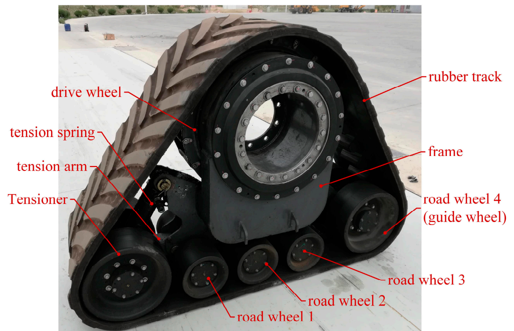
Figure 14. Physical prototype of high-speed rubber track assembly.
