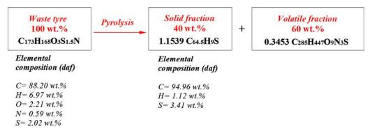
**Figure 6.** Elemental analysis of tire pyrolysis process (*daf* means dry ash-free basis) [6] (adapted with permission from Elsevier).
