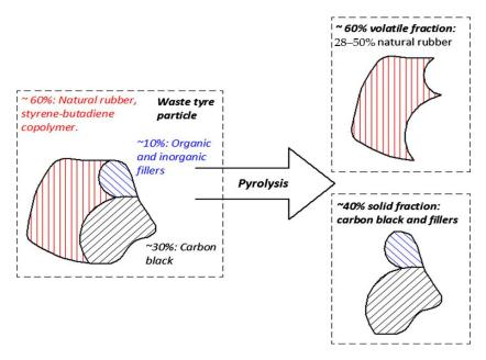
Figure 3. The scheme of WT pyrolysis [6] (Adapted with permission from Elsevier).
