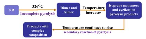
Figure 4. The pyrolysis process of NR.
