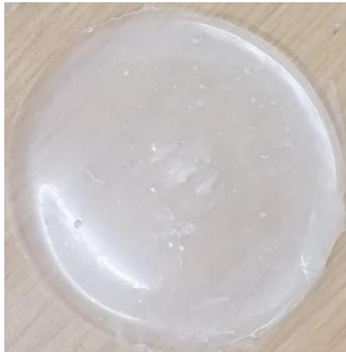
**Figure 2.** Snail shell nanoparticles and sugar bagasse cellulose fibers reinforced polylactic acid bioplastic film.
