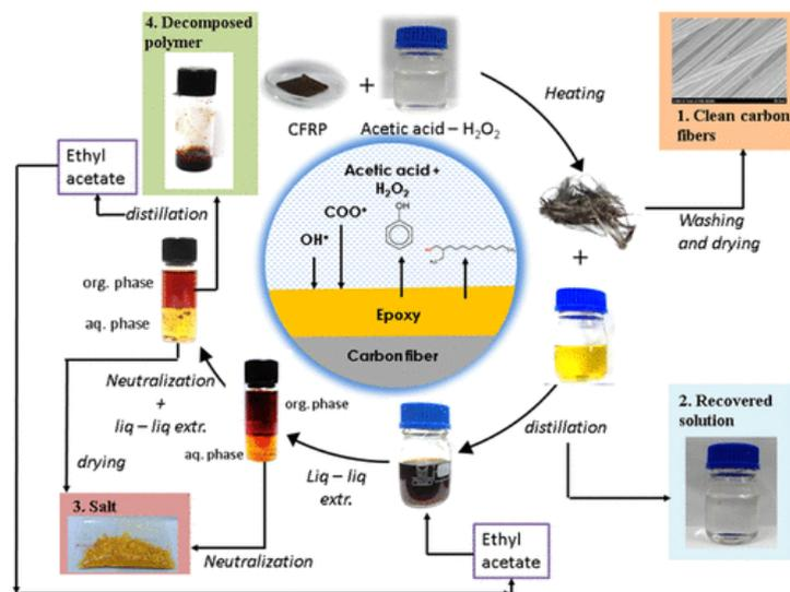
**Figure 9.** Schematic diagram of the green recycling process of CFRP. Reprinted with permission from Reference [161].
