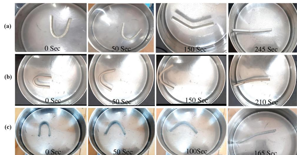
**Figure 11.** Shape recovery of (a) pure SMPU, (b) 0.5 wt% HNT-reinforced, and (c) 1% HNT-reinforced specimens at various time frames when placed in the water bath (at 80 °C).
