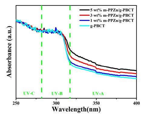
**Figure 5.** UV-Vis spectra of the g-PBCT and various weight ratios of g-PBCT/m-PPZn composites. The green lines in this figure illustrate the UV-A, UV-B, and UV-C regions.
