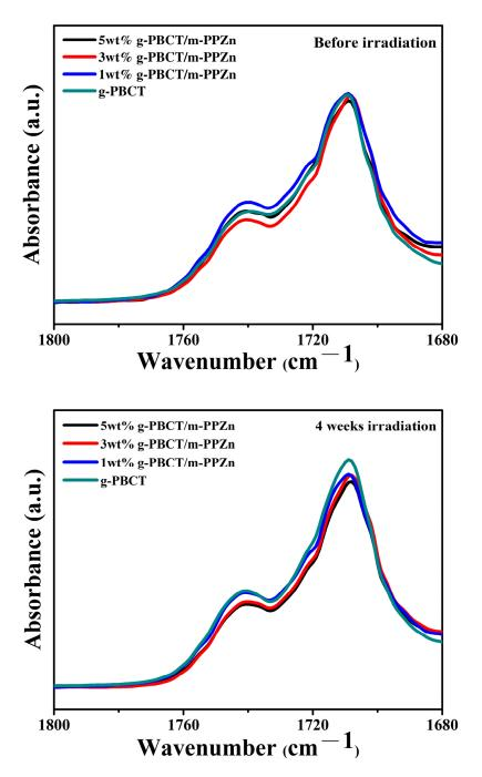
**Figure 7.** Change of FTIR spectra of g-PBCT and various weight ratios of g-PBCT/m-PPZn composites before and after 4 weeks UV irradiation times.
