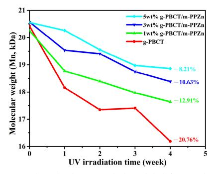
**Figure 9.** Change of number-average molecular weight (Mn) of g-PBCT and various weight ratio of g-PBCT/m-PPZn composites at different UV irradiation times.
