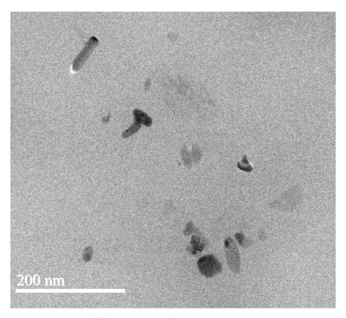
Figure 4. TEM images of the 5 wt% g-PBCT/m-PPZn composite.
