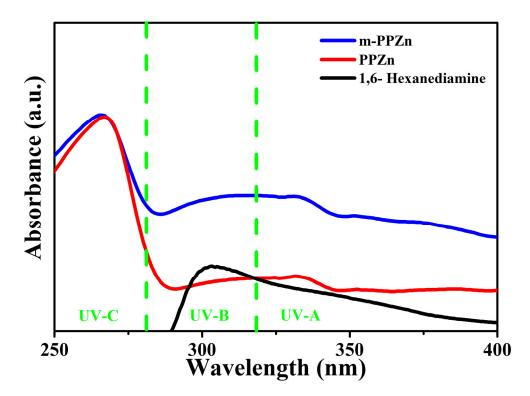
**Figure 2.** UV-Vis absorbance spectra of the PPZn, 1,6-hexanediamine and m-PPZn. The green lines in this figure illustrate the UV-A, UV-B, and UV-C regions.
