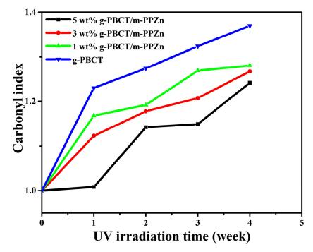
**Figure 8.** Change of carbonyl index of g-PBCT and various weight ratios of g-PBCT/m-PPZn composites at different UV irradiation times.
