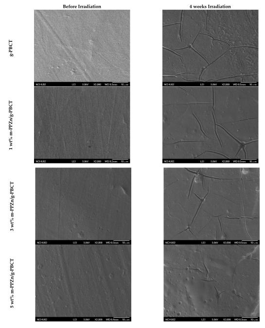
**Figure 10.** SEM images of g-PBCT and various weight ratio of g-PBCT/m-PPZn composites before and after 4 weeks UV irradiation times.
