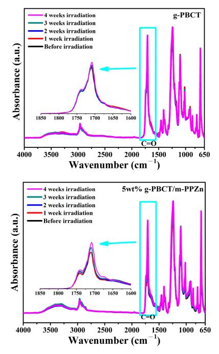
**Figure 6.** Change of FTIR spectra of g-PBCT and 5 wt% g-PBCT/m-PPZn composites nanocomposites at different UV irradiation times.
