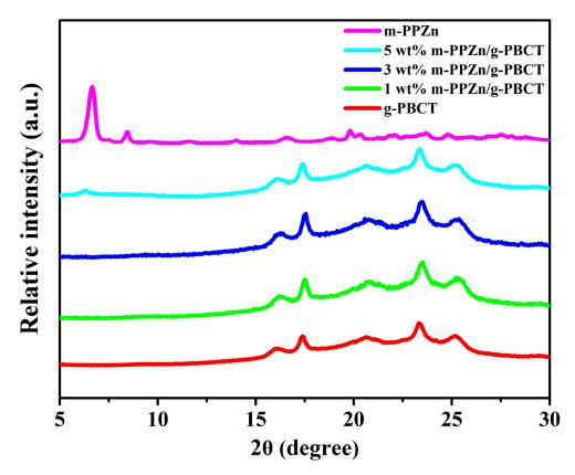
**Figure 3.** WAXD patterns of the m-PPZn, g-PBCT, and various weight ratios of g-PBCT/m-PPZn composites.
