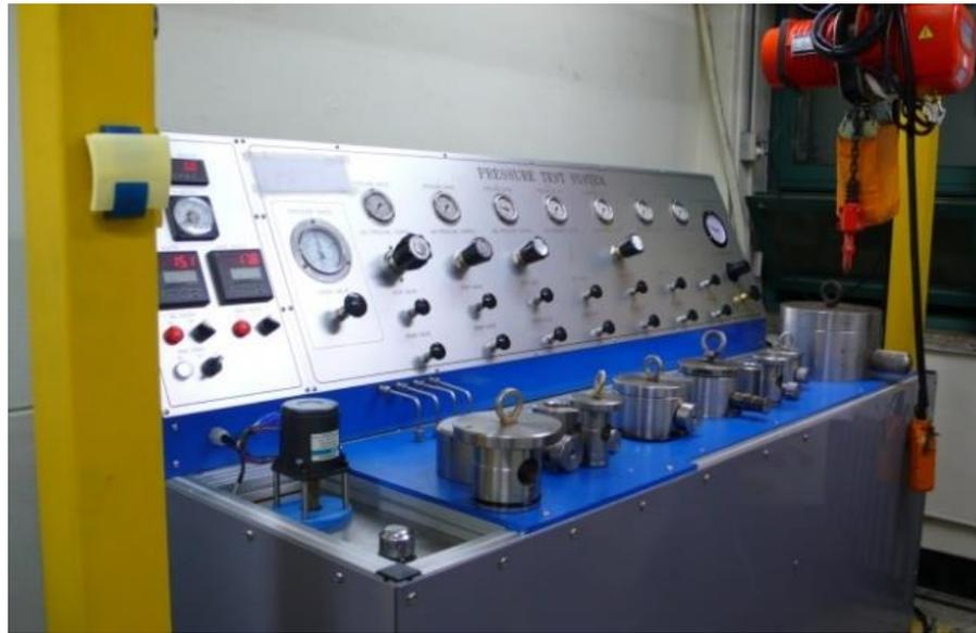
**Figure 2.** Experiment equipment for the solid-state batch-foaming process.
