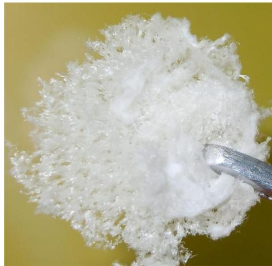
**Figure 5.** Photo of the obtaining MFC after freeze drying.
