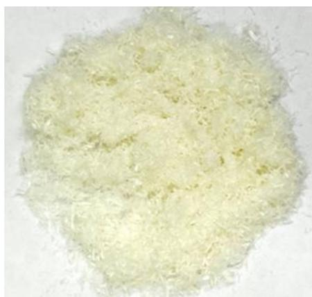
**Figure 1.** Cellulosic product obtained by peroxide delignification of spruce wood in the  $\text{CH}_3\text{COOH-H}_2\text{O}_2\text{-H}_2\text{O}$  medium over the sulfuric acid catalyst.
