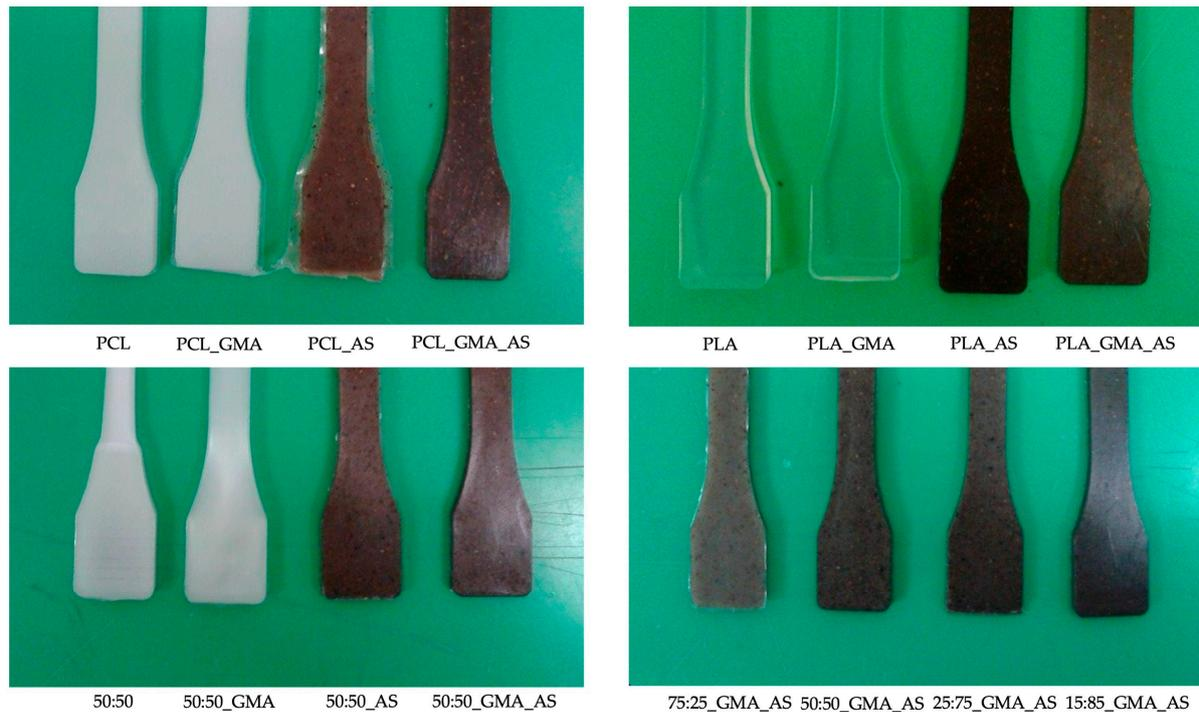
**Figure 1.** Visual appearance of the obtained biocomposites.
