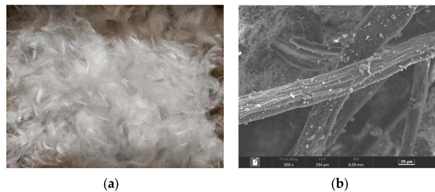
Figure 1. PE fiber: (a) Appearance; (b) SEM microtopography.
