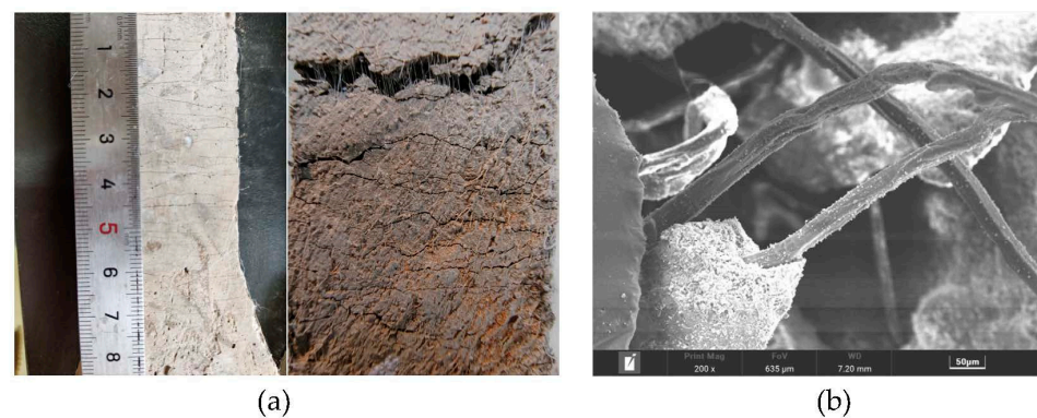
Figure 9. (a) Tensile crack distribution; (b) Microscopic morphology at the fracture.
