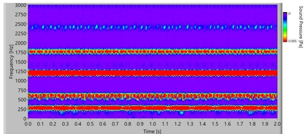
**Figure 14.** Frequency spectrogram of sound signal for polymer gears without coating.
