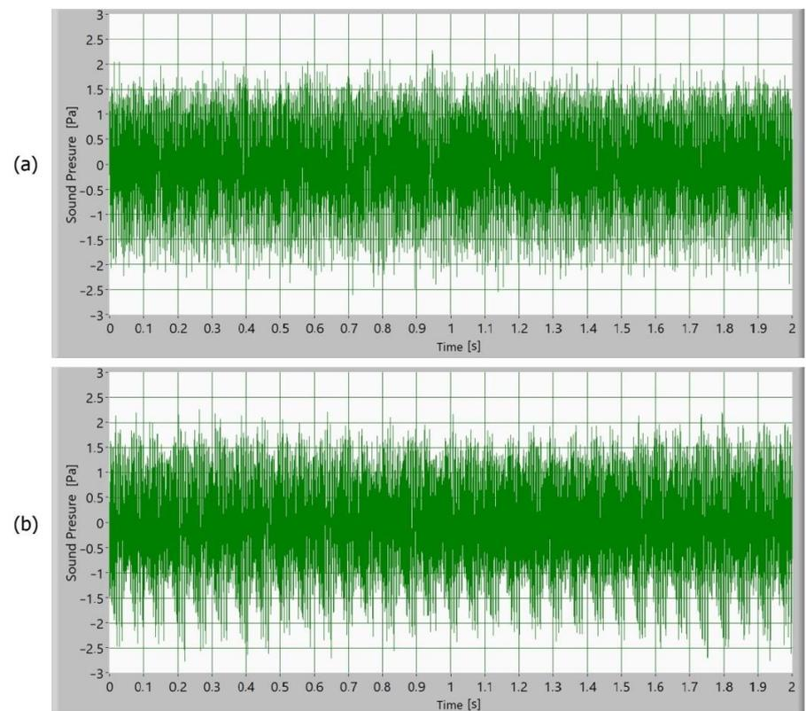
**Figure 8.** Time signal of sound pressure for polymer gears with CrN-coating with (a) 3-layer coating and (b) 5-layer coating.
