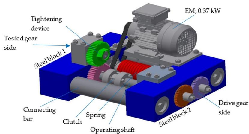
**Figure 3.** The principle of the testing device.
