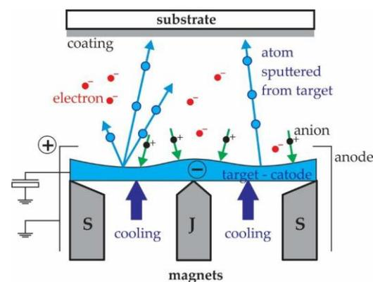
Figure 1. Magnetron sputtering process [1].
