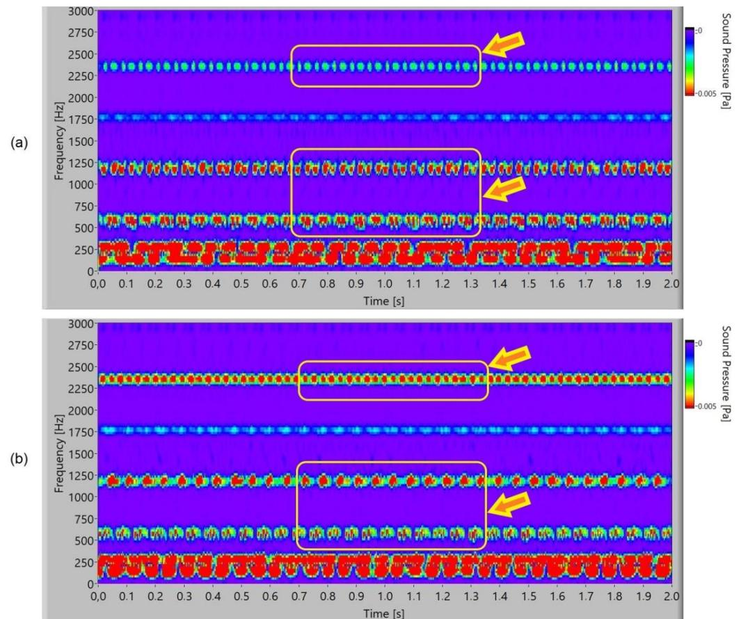
**Figure 17.** Frequency spectrogram of sound signal for polymer gears with CrN-coating: (a) 3 layers; (b) 5 layers.
