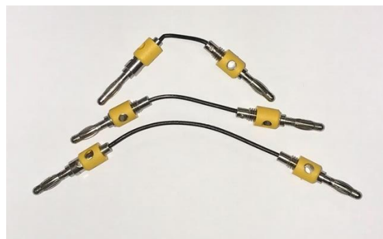
Figure 5. The 20, 40, and 80 mm test specimens connected to the banana probes.
